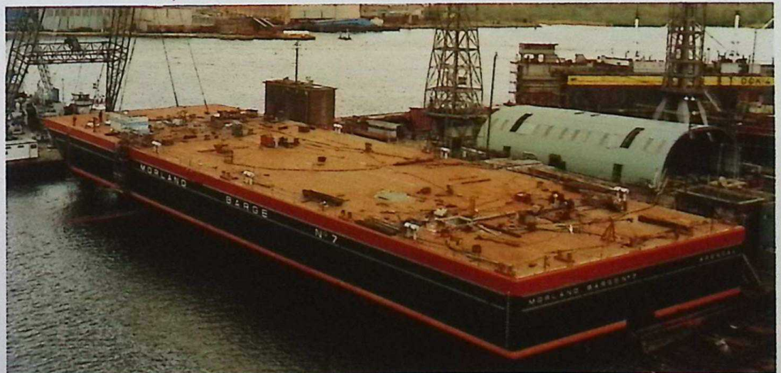
Two deck cargo barges of 91.5 × 27.4 × 6.1 metres were recently built for Arnt J. Mørland, Arendal, Norway. The photograph shows barge no. 7 on sideslip for welding of a butt.
