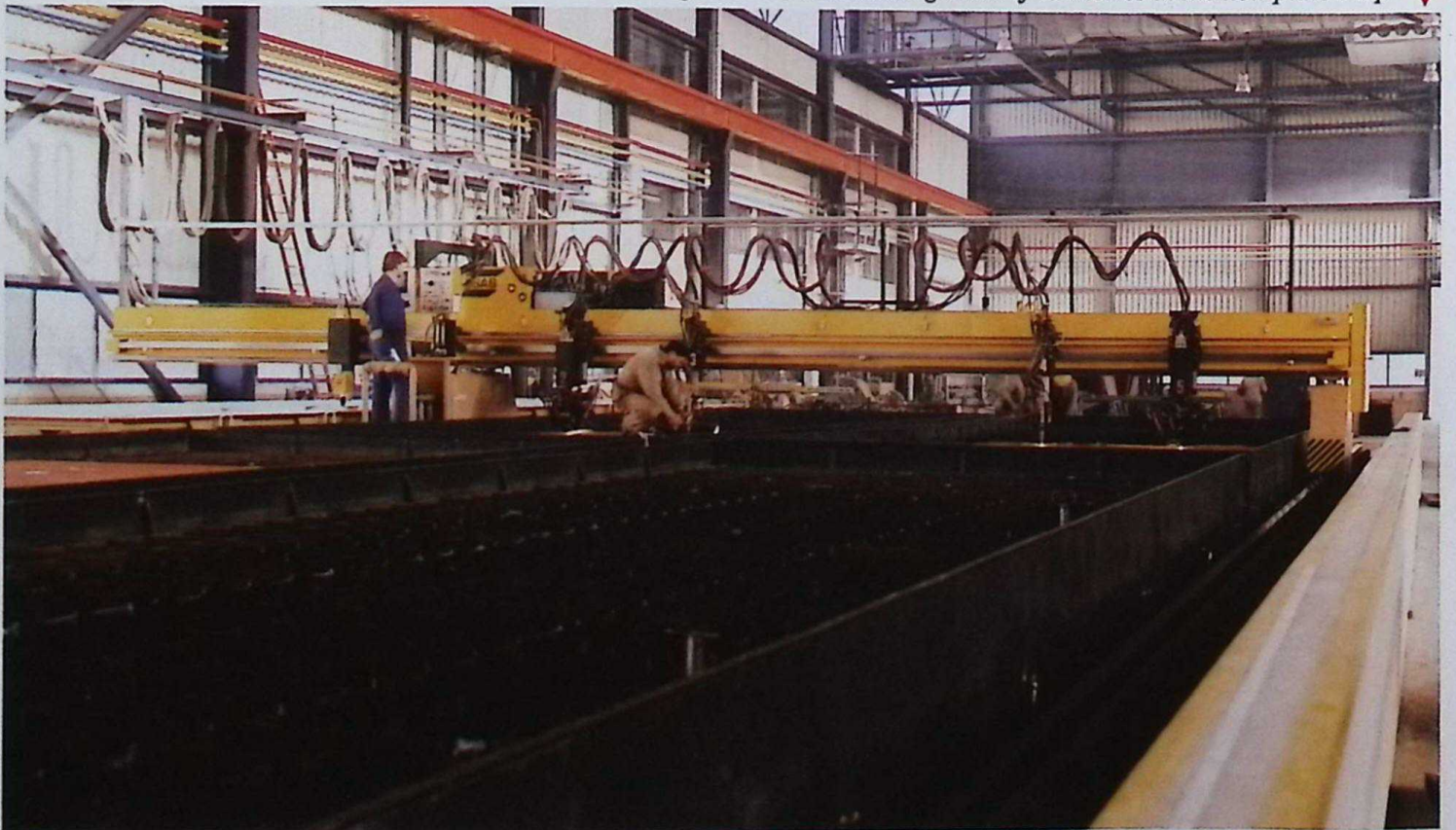
Flame cutting machine with running track of 28 metres in the new plate shop. ▼
